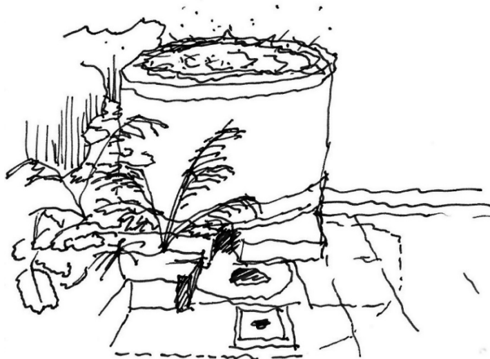
Fig. 26. As water reaches the dry well, it splashes out of the top while pooling at the base, Querini Stampalia, Venice, Italy, 1963.
